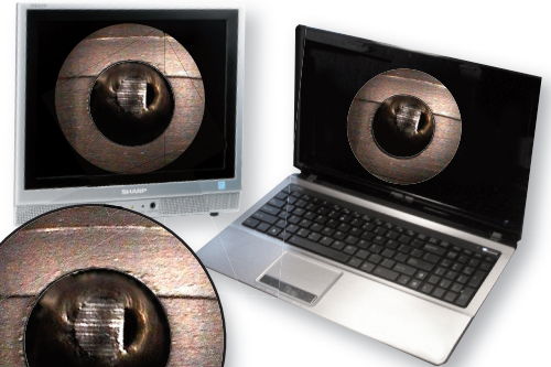
Blocked gas port viewed by eye, on a monitor, and on a computer.
